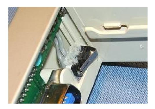
Pull the two wires through the space between the 50-pin plug at the back of the cradle and the rear face of the cradle, emerging close to the fan
