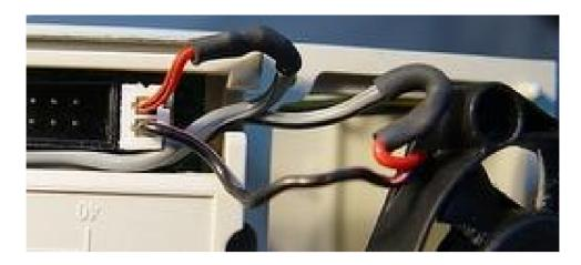
• Connect one of the emerged wires to one of the cut ends referred to in step 1, and the other emerged wire to the other cut end. The switch is then in series with the fan.
